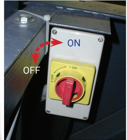
Drive Motor Disconnect Switch Figure 8-5
