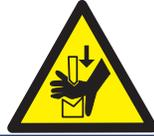
Pinch Hazard! Moving parts and pinch points are now exposed and can cause personal injury. Secure the area to prevent unauthorized access to the equipment before performing this maintenance step in accordance with the facilities' lockout/tagout program.
